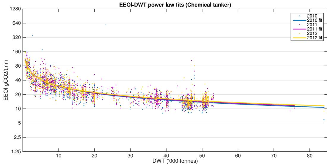
Figure 11: EEOI - dwt power law fits, chemical tanker
