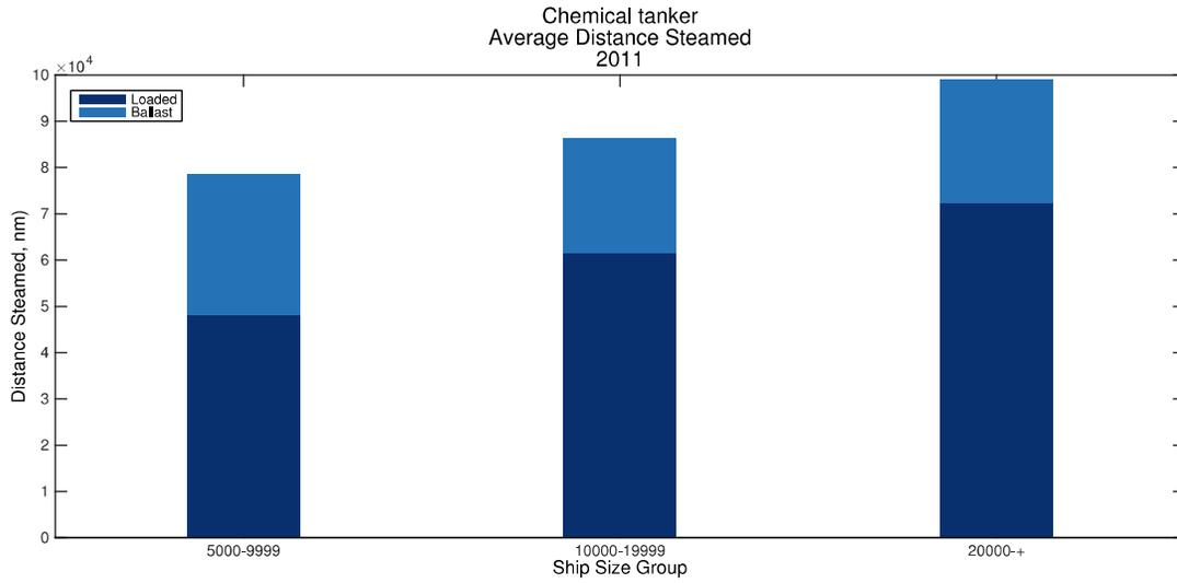
Figure 26: Data for the allocative utilisation as reported in noon reports for a small sample of chemical tankers
