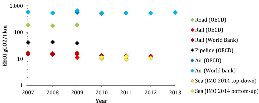
Figure 28: Top-down EEOI estimates for different modes of transport and years, using data from EIA (2010-14), OECD/ITF (2012), World Bank (2015), Smith et al. (2014) and data from this report (Table 9)
