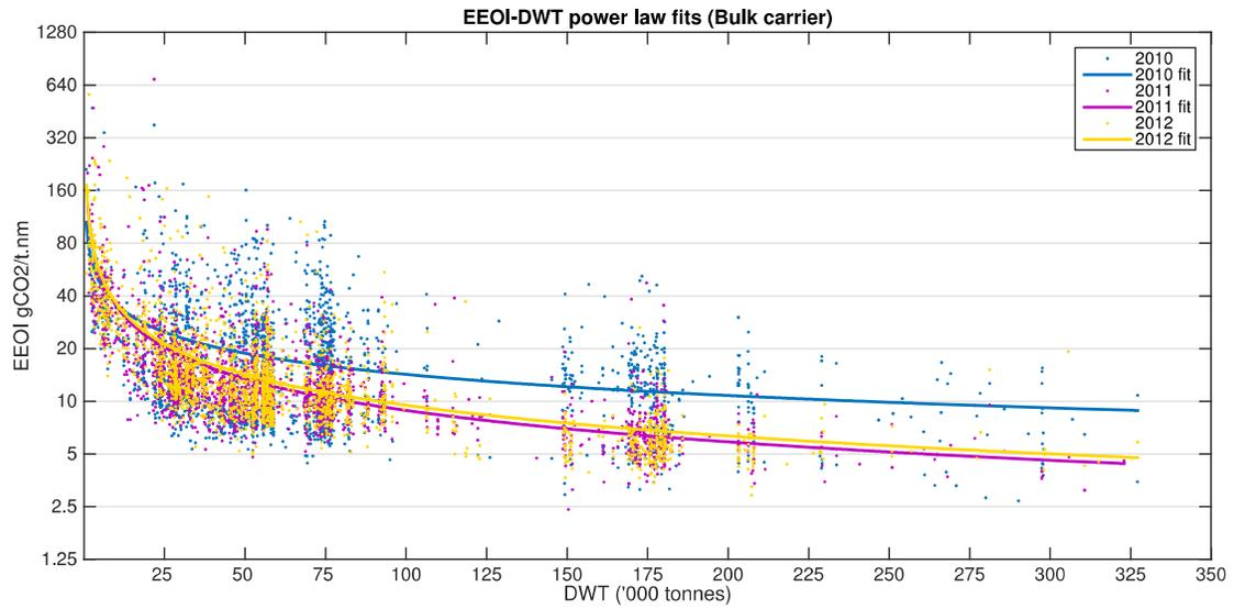
Figure 10: EEOI - dwt power law fits, bulk carrier
