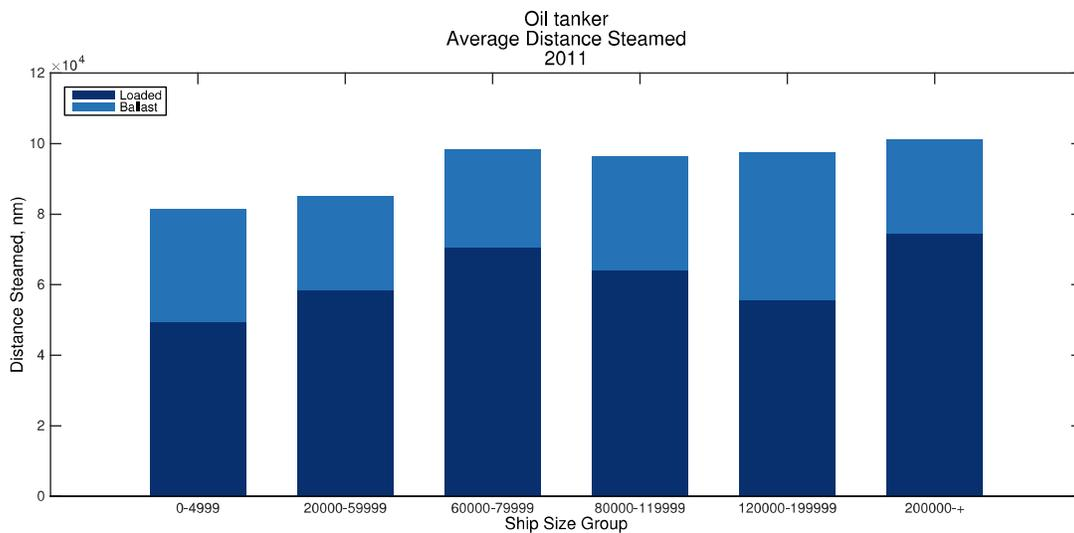
Figure 25: Data for the allocative utilisation as reported in noon reports for a small sample of oil tankers
