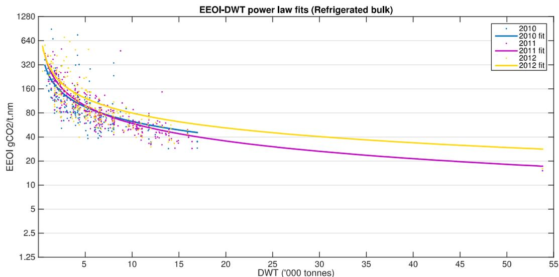
Figure 16: EEOI - dwt power law fits, refrigerated bulk
