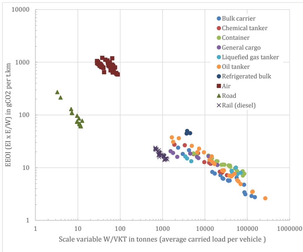
Figure 3: Comparison of EEOI for different modes of transport
