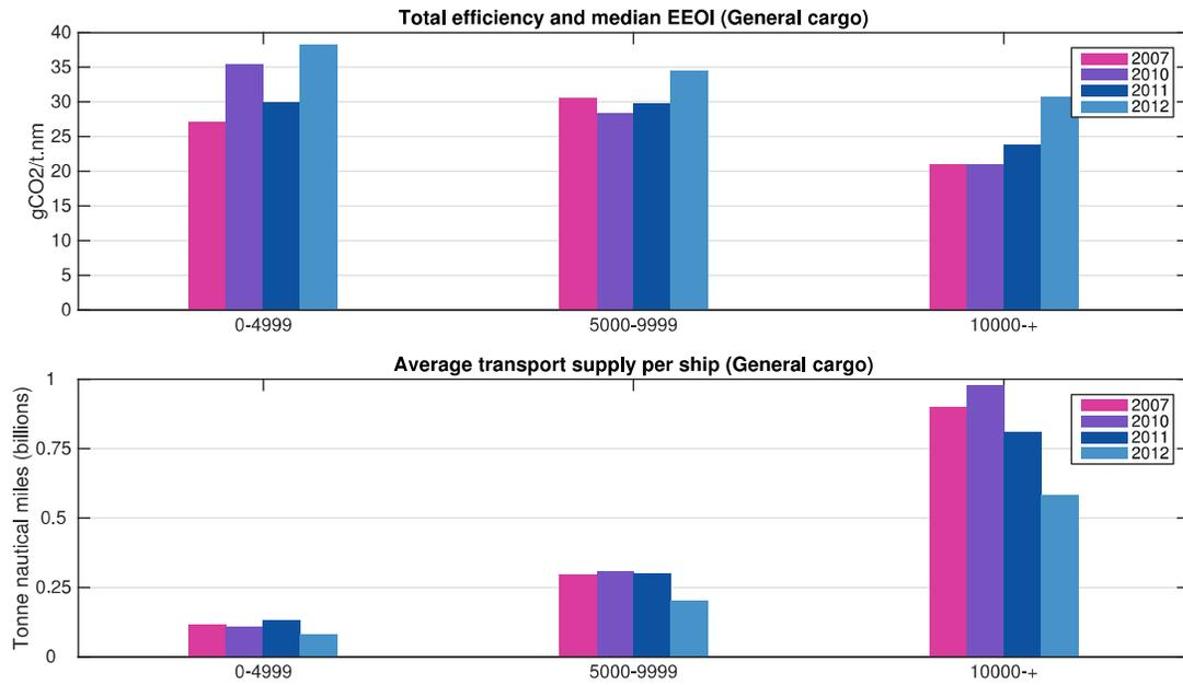
Figure 8: EEOI and transport supply 2007 to 2012, general cargo
